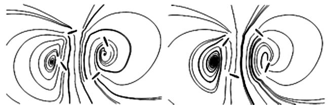
Fig. 9 Instantaneous streamlines in the symmetry plane of the rotor for two consecutive rotor positions.
